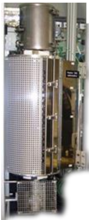
reactor with tubular furnace and insulation
