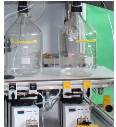
Liquid dosing with HPLC pumps
