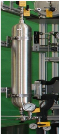
Liquid gas tank
