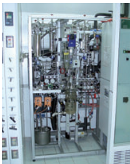
3-litre glass plant for 3 bar
