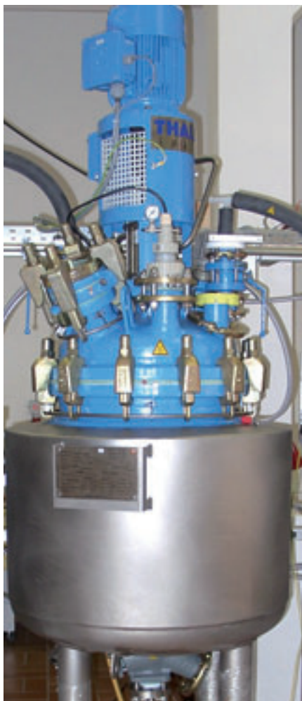
Glass lined steel reactor (100 litre)
