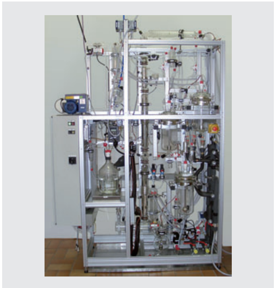
Automated continuous rectification plant with Sulzer™-packing, Ø 30 mm, with phase separator, completed with all necessary measurements and control instruments (Dimensions W x D x H = 1500 x 800 x 2300 mm)
