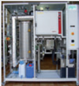
Catalyst testing unit with two reactors, 750 °C, 40 bar
