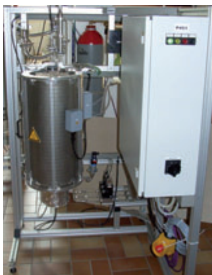
Tubular reactor, 1000 °C
