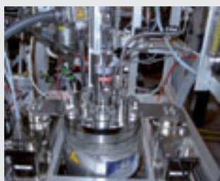
Lid of a 2 l reactor on compensated load cells
