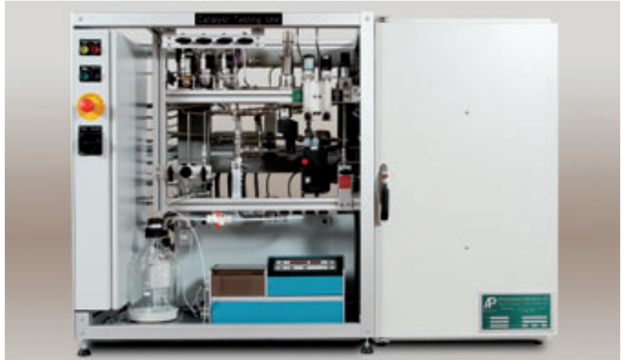
Bench-top micro reactor system for catalyst testing Dimensions W x D x H = 1400 x 490 x 980 mm
