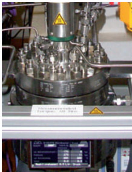
Stirred vessel, 175 bar
