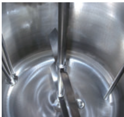
Stainless steel reactor inside
