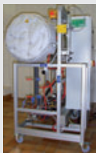
Extraction unit for plastic pellets, vacuum, 250 °C
