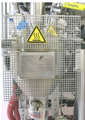
Reactor with safety guard
